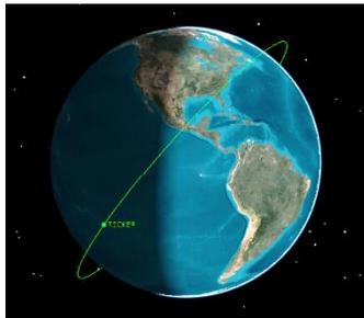
The spacecraft is to be launched into a circular orbit at an altitude of 1,000 kilometers (621 miles) and an Inclination of 50°. **TICKER 2** will have an orbital period of 105.119 minutes, so it will orbit the Earth 13.7 times in 24 hours. This orbit will allow the satellite to contact each of the many world Stock Exchange locations several times each day and will allow a significant amount of data to be received from and shipped to each of the Exchanges.
