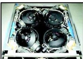
To insure that **TICKER** successfully transmits and receives data from the ten Stock Exchanges, the satellite must maintain a very stable and precise orientation. The spacecraft accomplishes this by using control moment gyroscopes to keep the satellite
